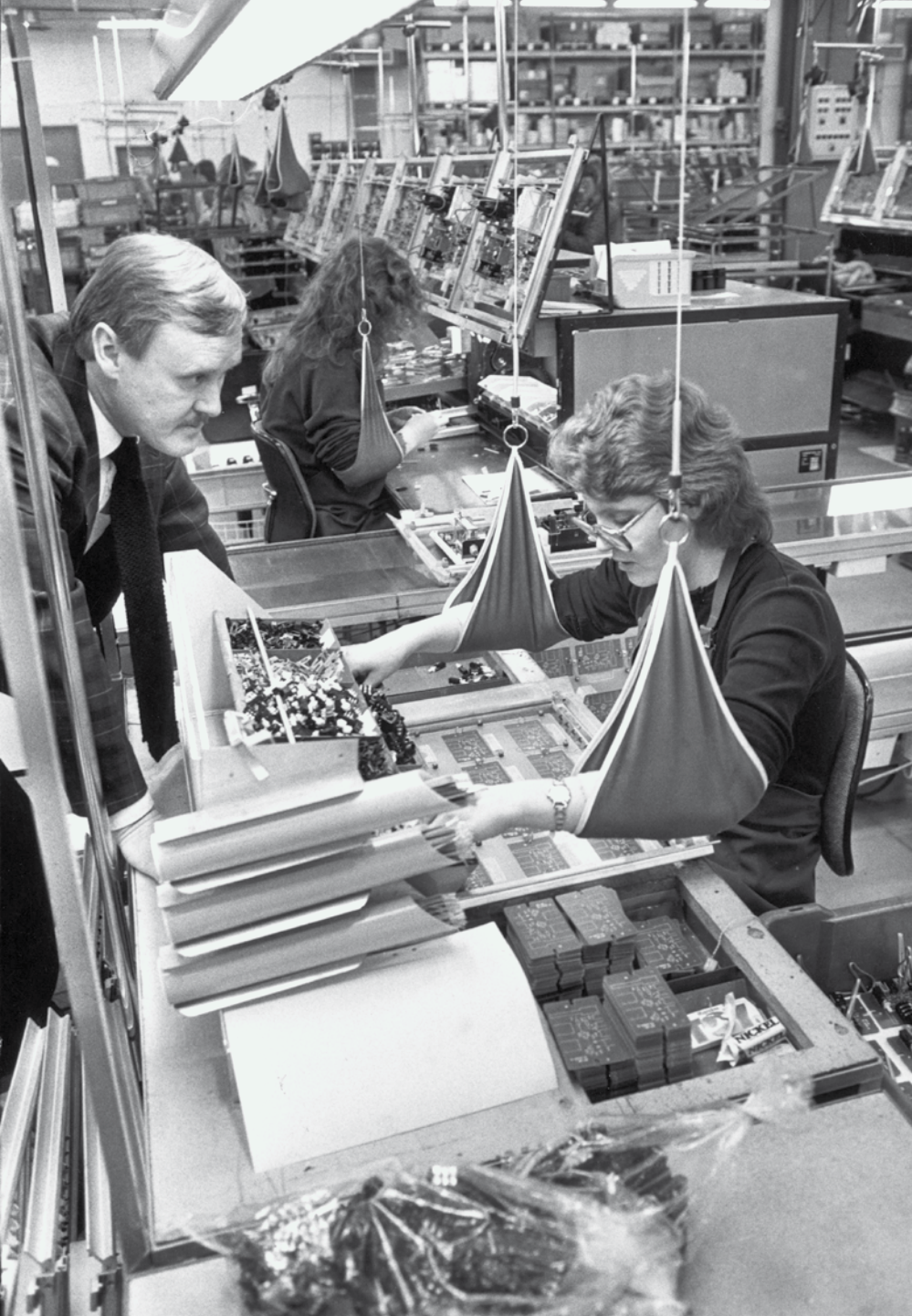
Assembly work at the Luxor factory in Norrköping in 1985. To avoid repetitive strain injuries to arms and shoulders, the women have both arms in a sling.
